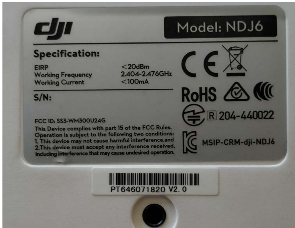
Figure 3: Working frequency of DJI Phantom 2 transmitter
